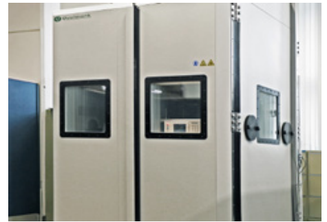
Highly Accelerated Life Testing Equipment
